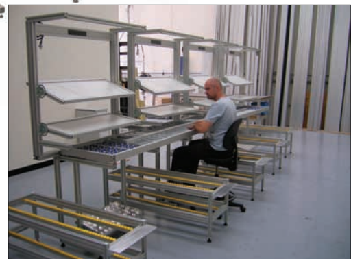
15. manual assembly line with gravity conveyors
